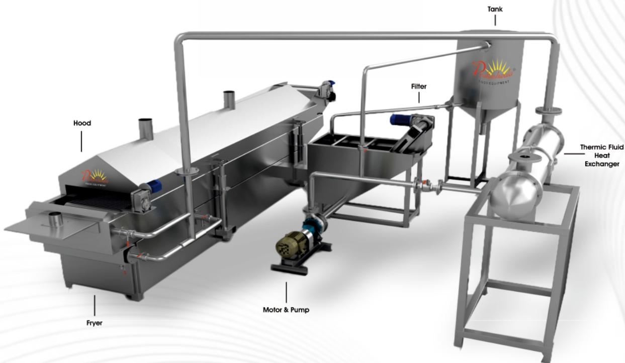
THE MULTI PRODUCT CONTINUOUS FRYING SYSTEM IS AN ARRANGEMENT, WHICH IS SUITABLE FOR FRYING OF VARIETY OF SNACKS.
